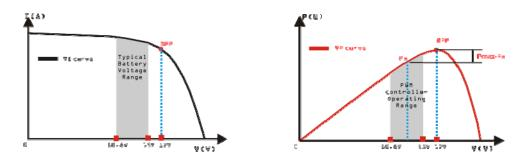
Nominal 12 Volt Solar Module I-V curve and output power graph
